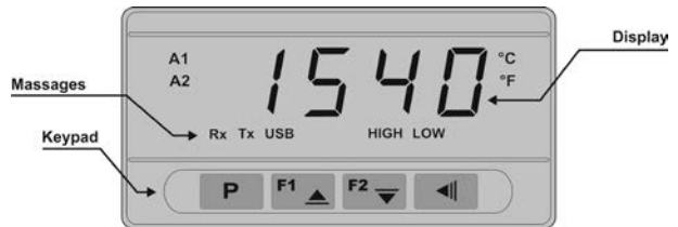
Figure 02 - Identification of the front panel parts
